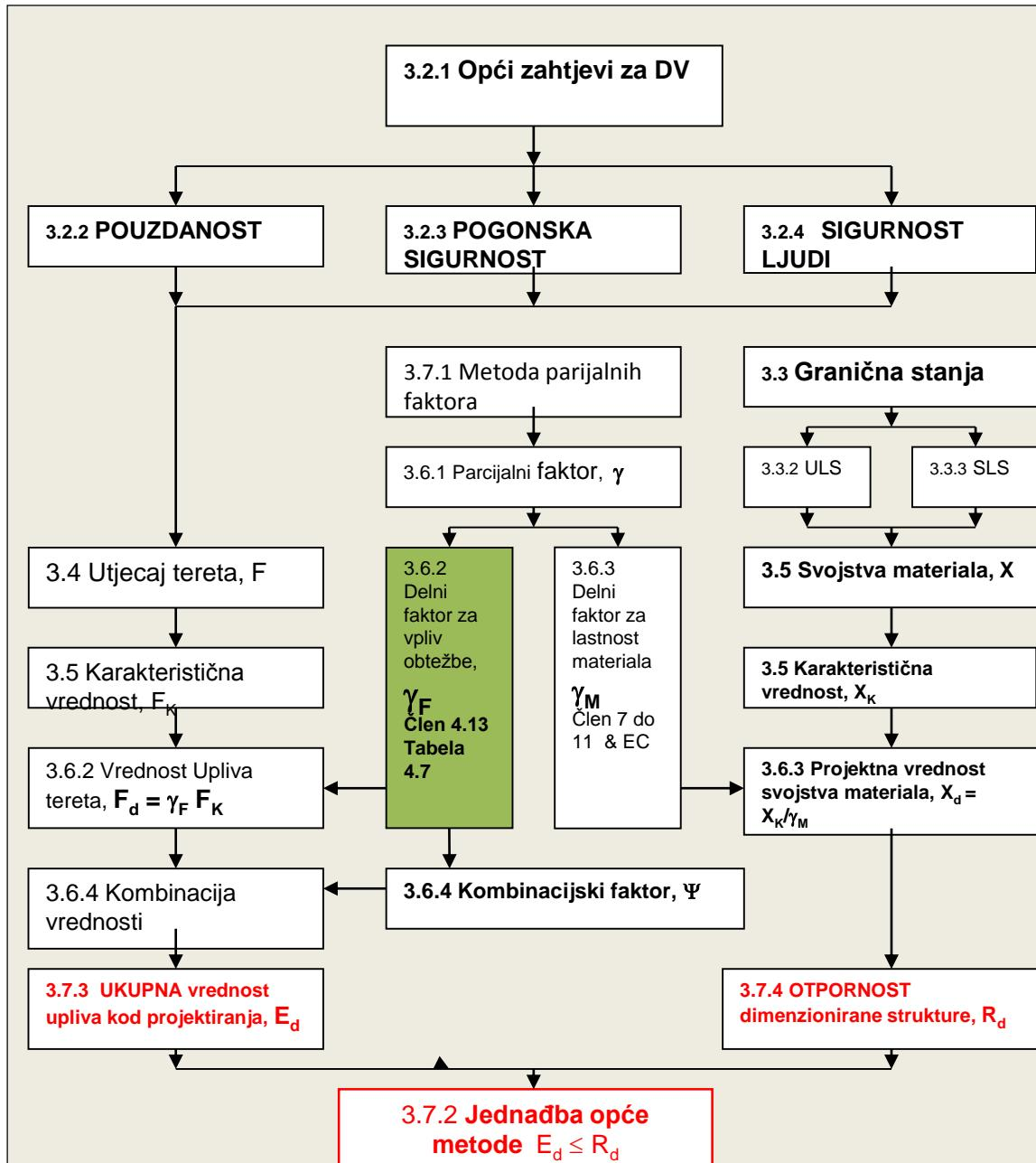
**Reliability requirements** are achieved by design according to: **EN 50341-1, EN 1990, EN 1991** and **EN 1993**. Minimum reliability level 1 for overhead lines, i.e., the return period  $T$  of climatic actions is 50 years.
