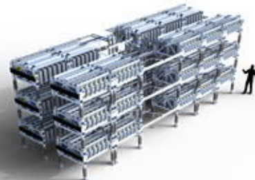
+/-30kVdc, 90MW Converter Tower
